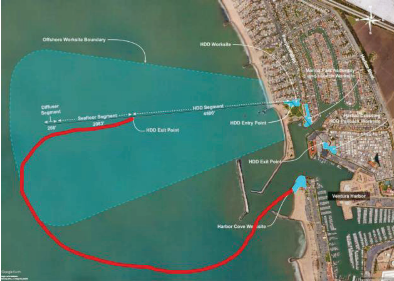
Seafloor Segment HDPE Pipeline pull-out route
