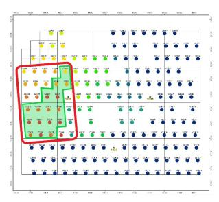
The area outlined in red indicates the focus over the next 2-3 weeks. The green area indicates completed monopile installations as of June 17, 2024. Monopile installation will follow a general clockwise pattern around the lease area.
