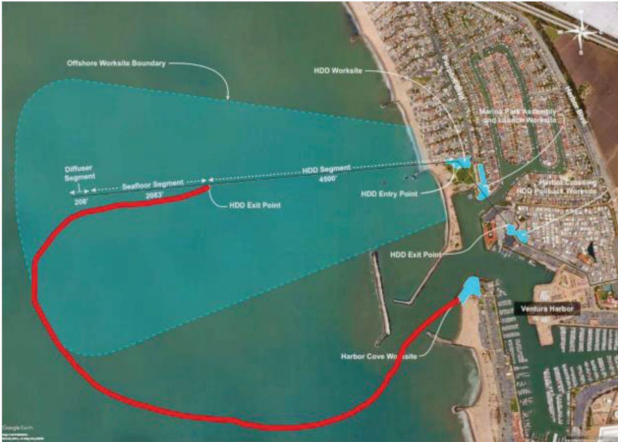
Sea floor Segment HDPE Pipeline pull-out route
