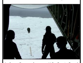
Iceberg Reconnaissance: U.S. Coast Guard fixed-wing aircraft equipped with radar operate out of St. John's, Newfoundland during the ice season to conduct the primary reconnaissance for the Ice Patrol. Aircraft also deploy oceanographic equipment such as drifting buoys to obtain real-time ocean current and sea surface temperature data.
