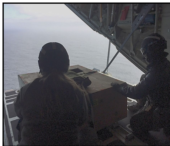
Figure 4-2. Aircrew preparing to deploy the last of IIP's aerial deployable 50m SVP buoys during a patrol on 11 May 2019.
