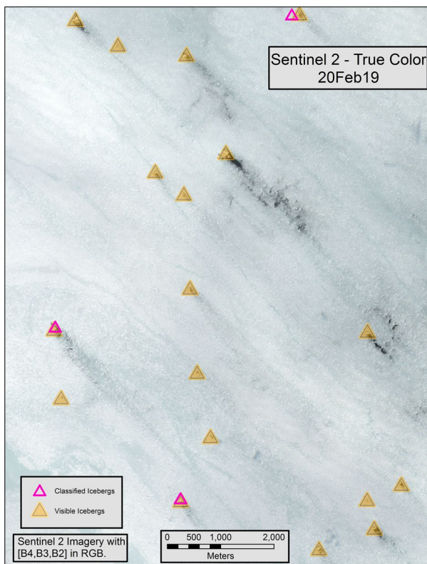
Figure B-7. Subset Sentinel-2 true color image from 20 February 2019. Here, three SDW classified icebergs from the SAR image (pink triangles) are compared with the 18 verified icebergs in the true color image (orange triangles). In this subset, the three SAR classified icebergs were accurately identified, however, the 15 false negatives shown here highlight the challenges that still exist with identifying icebergs within sea ice.
