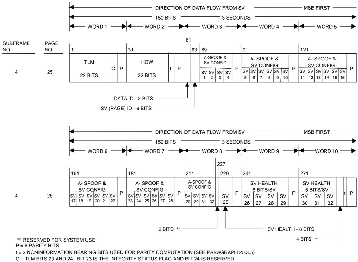
Figure 20-1. Data Format (sheet 9 of 11)
