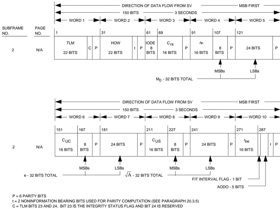
Figure 20-1. Data Format (sheet 2 of 11)
