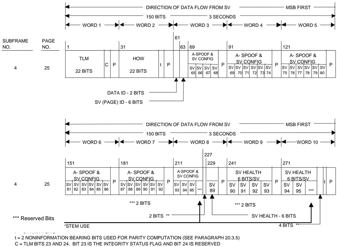
Figure 40-1. Data Format (sheet 9 of 11)
