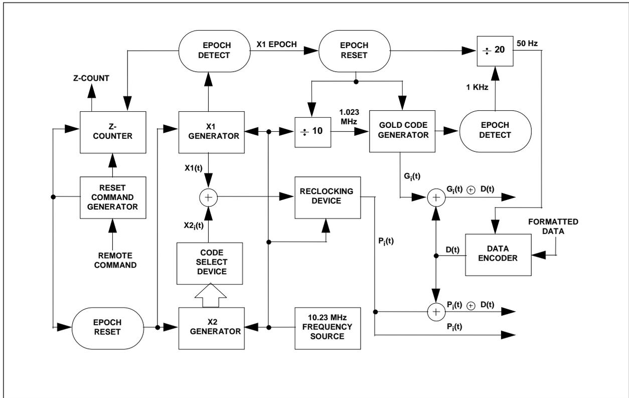
Figure 3-1. Generation of P-, C/A-Codes and Modulating Signals
