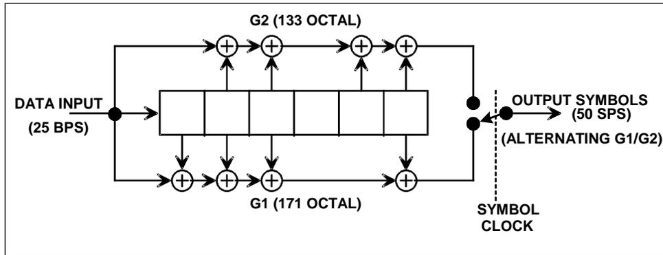
Figure 3-14. Convolutional Encoder
