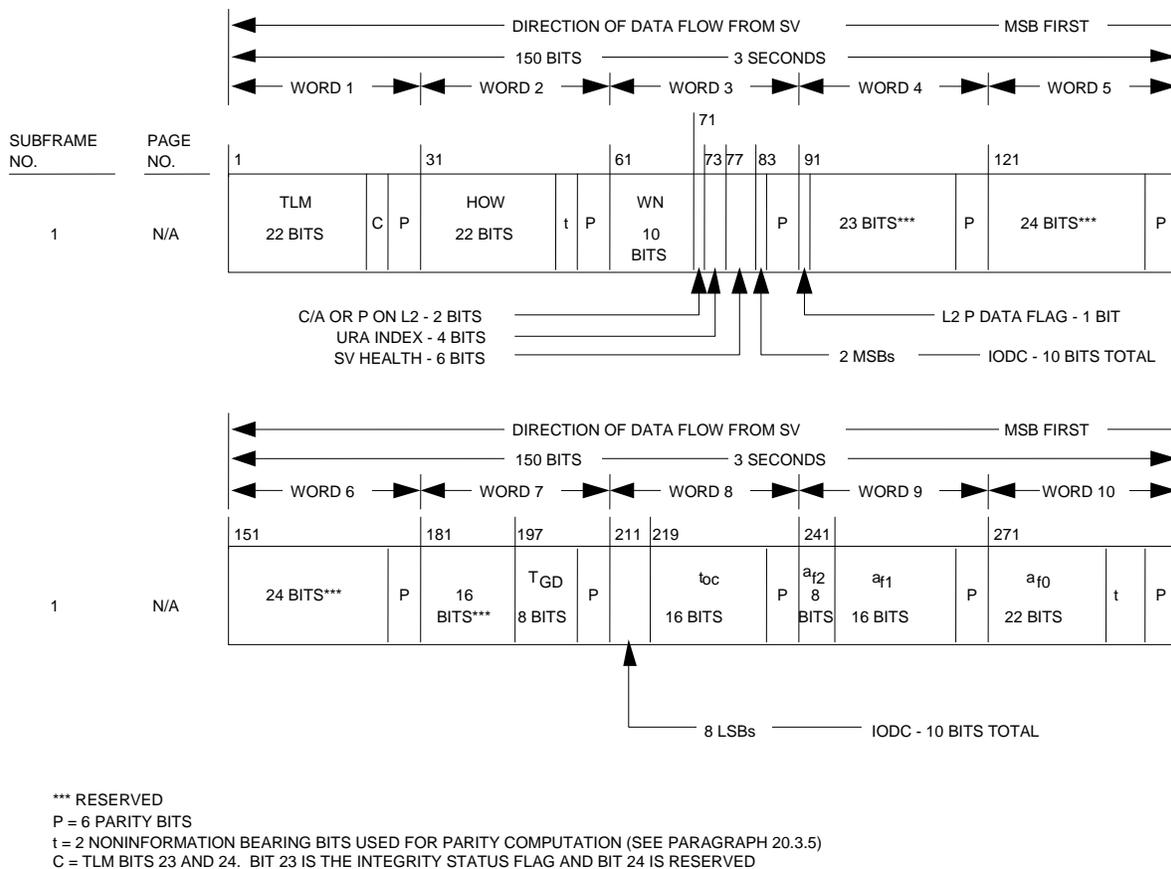
Figure 20-1. Data Format (sheet 1 of 11)
