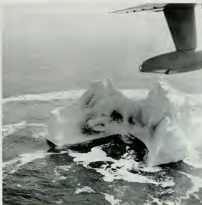
Figure 2. Photo taken minutes after a strike by a 1000-lb bomb during the 1960 tests. The bomb caused a spray of ice fragments, but no significant change in the iceberg's shape.
