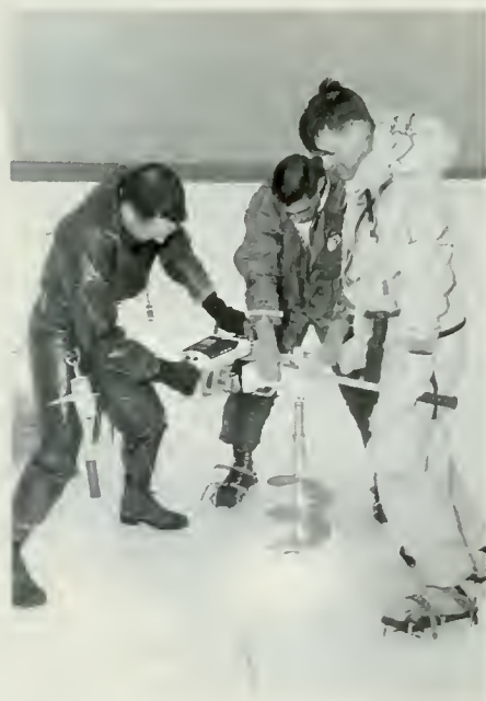
Figure 3. Drilling a hole in the iceberg with a power auger was a 45-minute procedure
